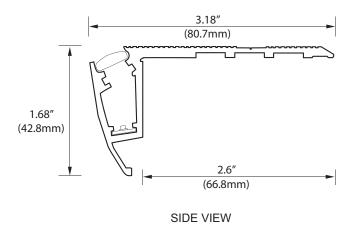
Impact Lighting's **XTRU-4810** Topline Series Step Lighting is an aluminum stair profile with LED tread illumination with single or RGB color options. Perfect for theater applications this profile offers an optional lighted aisle marker with number, letter or symbol.
