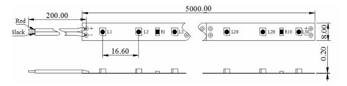
NOTE: 1. All dimensions are in millimeter. 2. Tolerance of measurement is  $\pm 0.05$ mm (.02") unless others otherwise noted.
